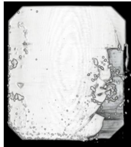
A CT scan of a body armor plate.
