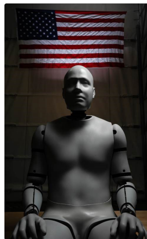
WIAMan ATD developed for live-fire testing in UBB events.
